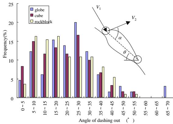
Figure-14. Beginning flight angle after it collides(all cases)
