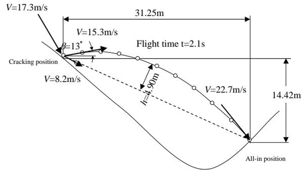
Figure-20. Beginning flight from gentle inclination part      Figure-21. Flight movement of cracking concrete ball
