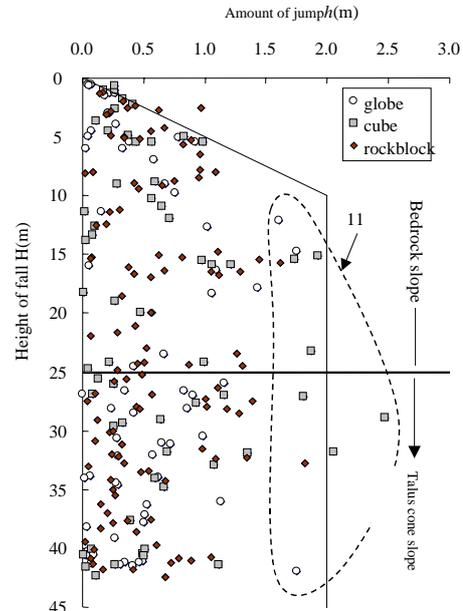
Figure-18. Amount of jump of falling rock
