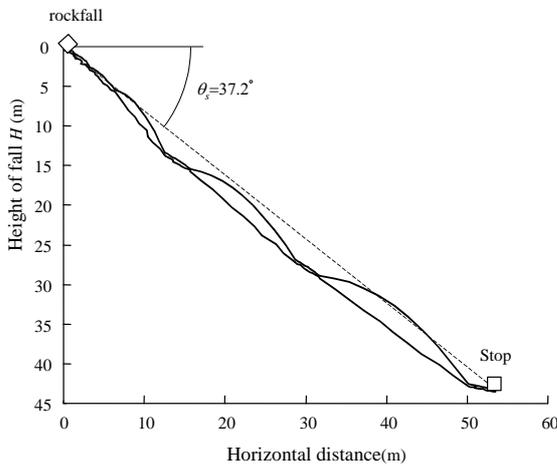
Figure-9. Cubic block vertical through fall route (After deforesting the tree.)
