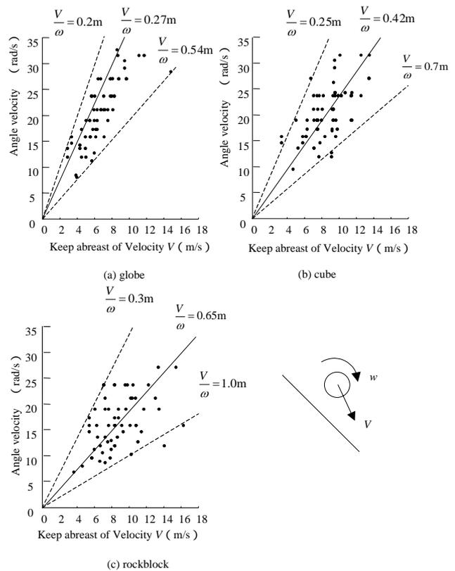
Figure-15. Relation between keep abreast of velocity and corner velocity
