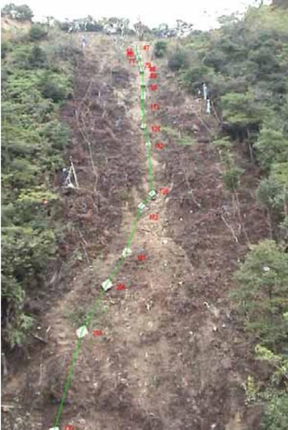
Photograph-3. Cubic block fall situation(After deforesting the tree. )
