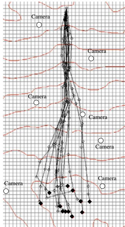
Figure-7 Plane surface fall route of rockblock
