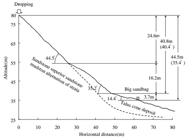
Figure-3. vertical of experiment slope
