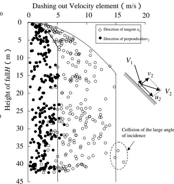
Figure-13. Beginning flight speed element after it collides (all cases)
