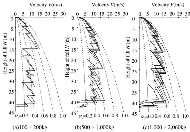
Figure-12. Mass and keep abreast of velocity of falling rock(After deforesting the tree. rockblock)
