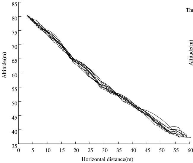
Figure-8. vertical through fall route of falling rock (After deforesting the tree.)
