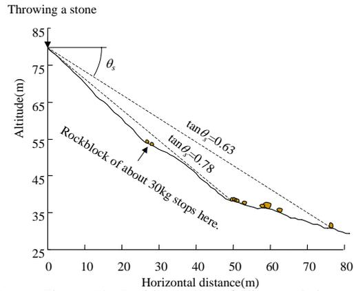
Figure-10. Position where falling rock in preliminary experiment is stopped(Before the tree of deforestation, rockblock)
