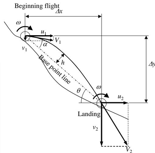
Figure-4. Explanation of sign the rockblock in the experiment.
