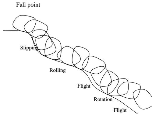
Figure-6. Pattern diagrams in movement form of rockblock
