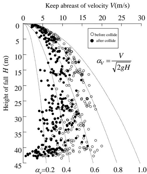
Figure-11. Relation between fall amount and keep abreast of velocity(all cases)
