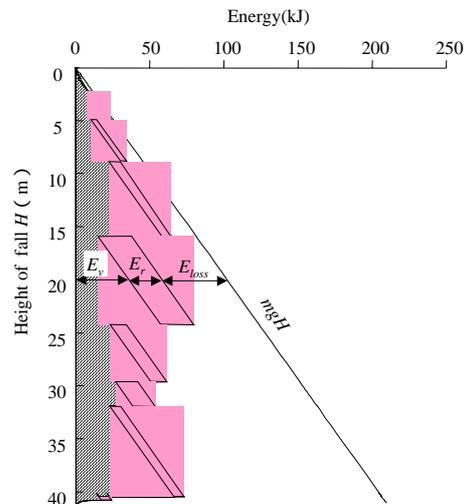
Figure-16. Change in energy of falling rock (After deforesting the tree. Cubic block)
