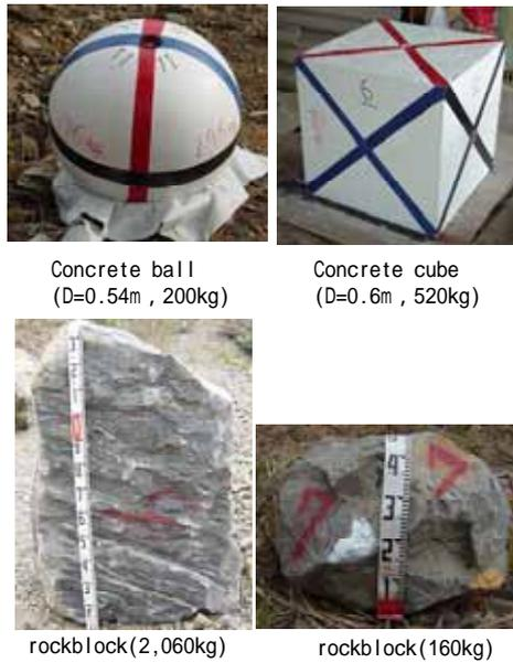
Photograph-2. Falling rock used to experiment
